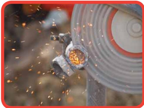
The ALTRAD Belle specialist range of Diamond Blades has a 10mm or 12mm high segment with high diamond concentration. The PUX range is the ultimate multi purpose diamond blade.
