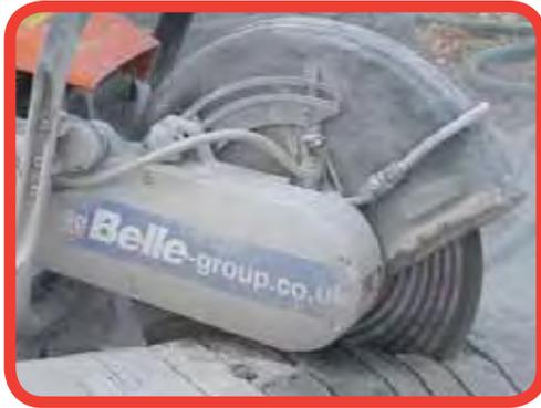
ALTRAD Belle's Platinum range of Diamond Blades has a double laser welded 10mm high diamond segment. These have been designed to give excellent speed of cut and a very long life. Excellent value for money. ALTRAD Belle's Gold and Bronze range of Diamond Blades are designed to provide good productivity levels at the lowest possible cost. There is a blade to suit everyone's needs.
