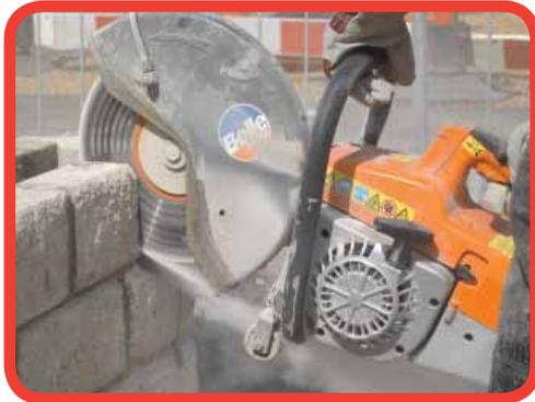
The Gold range of 10 - 15mm high segment double laser welded diamond products is a range of high quality blades specifically designed to provide good productivity levels at the lowest possible cost. Blades 300mm and over include 15mm undercut protection-segments.
